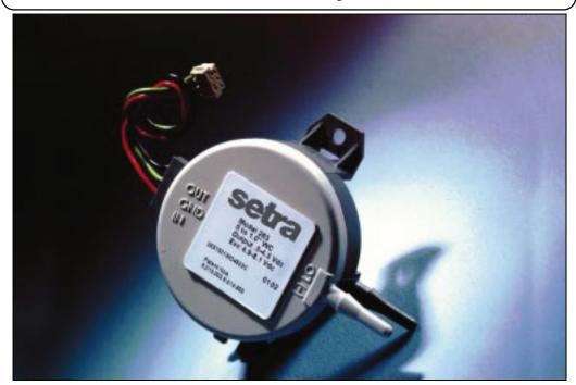
etra Systems Model 263 pressure transducers sense differential or gauge (static) pressures and convert this pressure difference to a proportional electrical output. The 263 is offered with a high level 5 VDC output.
